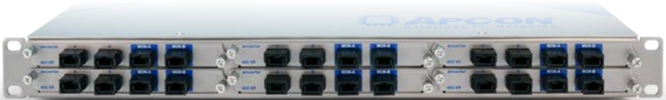
40G SR TAP Chassis (6 Modules)
