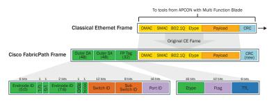
APCON's Multi Function blade performs protocol stripping on any port, up to 288 1G or 10G ports in an 8RU chassis.
