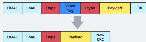
APCON's IntellaView performs protocol stripping on any port, up to 288 40G or 100G ports in a 9RU chassis.
