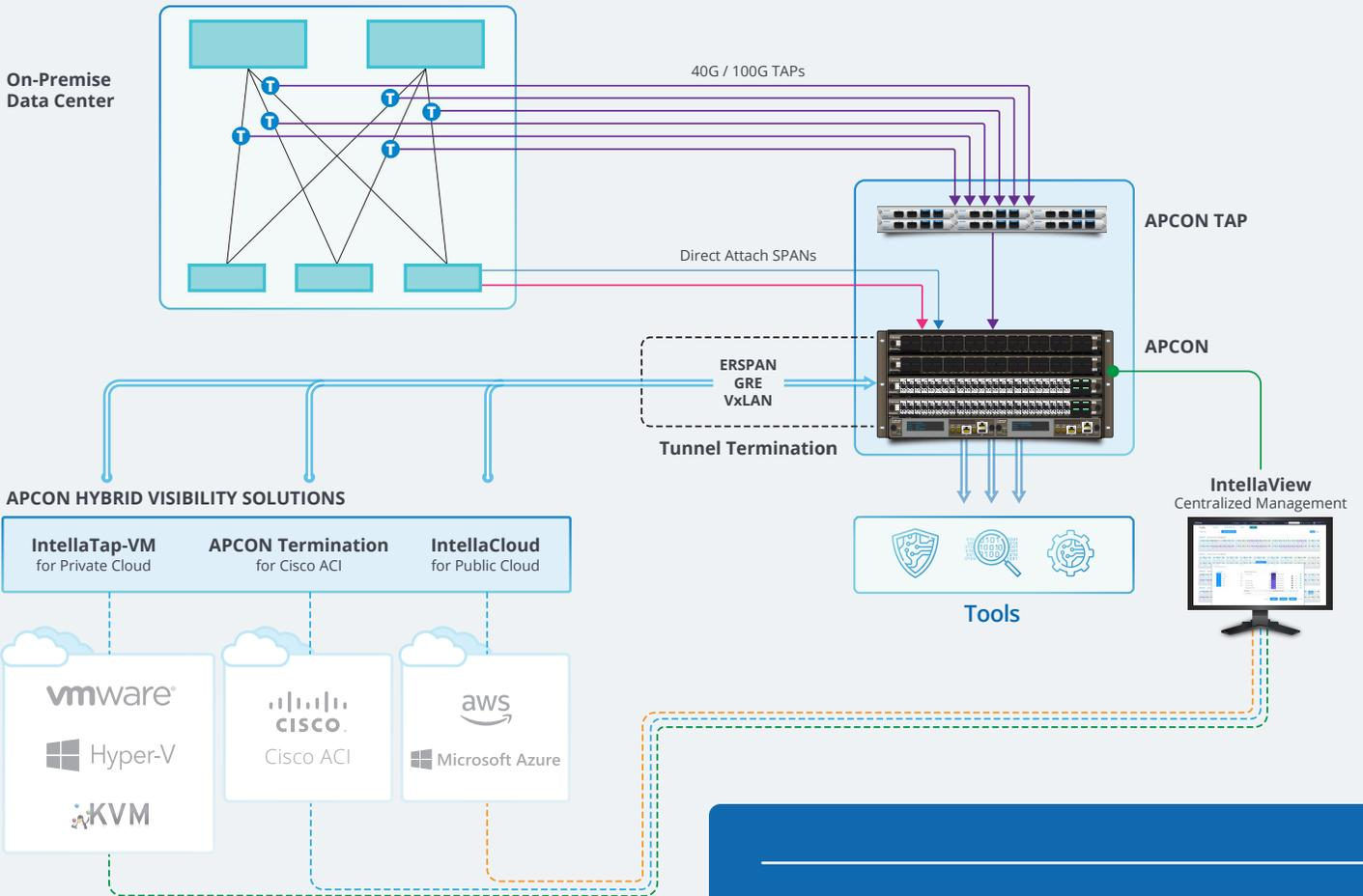
IntellaView is part of APCON's hybrid network visibility solution which also includes IntellaTap-VM and IntellaCloud, providing tunnel termination to monitor high-speed, high-volume traffic of interest.
